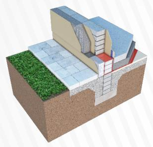
KORE External is a high performance expanded polystyrene (EPS) insulation board that is used in conjunction with a composite external thermal insulation system. The product consists of rigid boards cut from moulded blocks of EPS. The blocks are aged for four to six weeks to ensure the product is delivered to site to the exacting tolerances required for external insulation products. KORE External products are available in two grades of material, silver and white, and a range of thicknesses.
